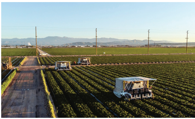
Advanced Farm's robotic harvesters drive autonomously over strawberry beds. One harvester can pick 100 pounds of strawberries per hour.
