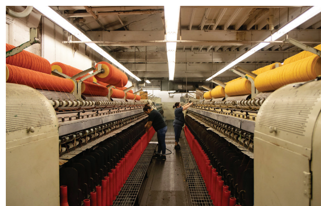
Employees at Pendleton Woolen Mills in Pendleton, Ore., work beside spinning frames, which take the wool from the roving stage to the yarn stage by simultaneously drafting or stretching the roving and twisting. This process entraps the fibers and gives the yarn strength and a defined texture.
