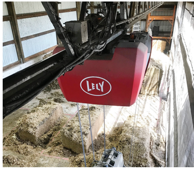
A bridge crane scoops a load of silage from the feed kitchen to be mixed and delivered via robot to dairy cows at Tilla-Bay Farms in Tillamook, Ore.
