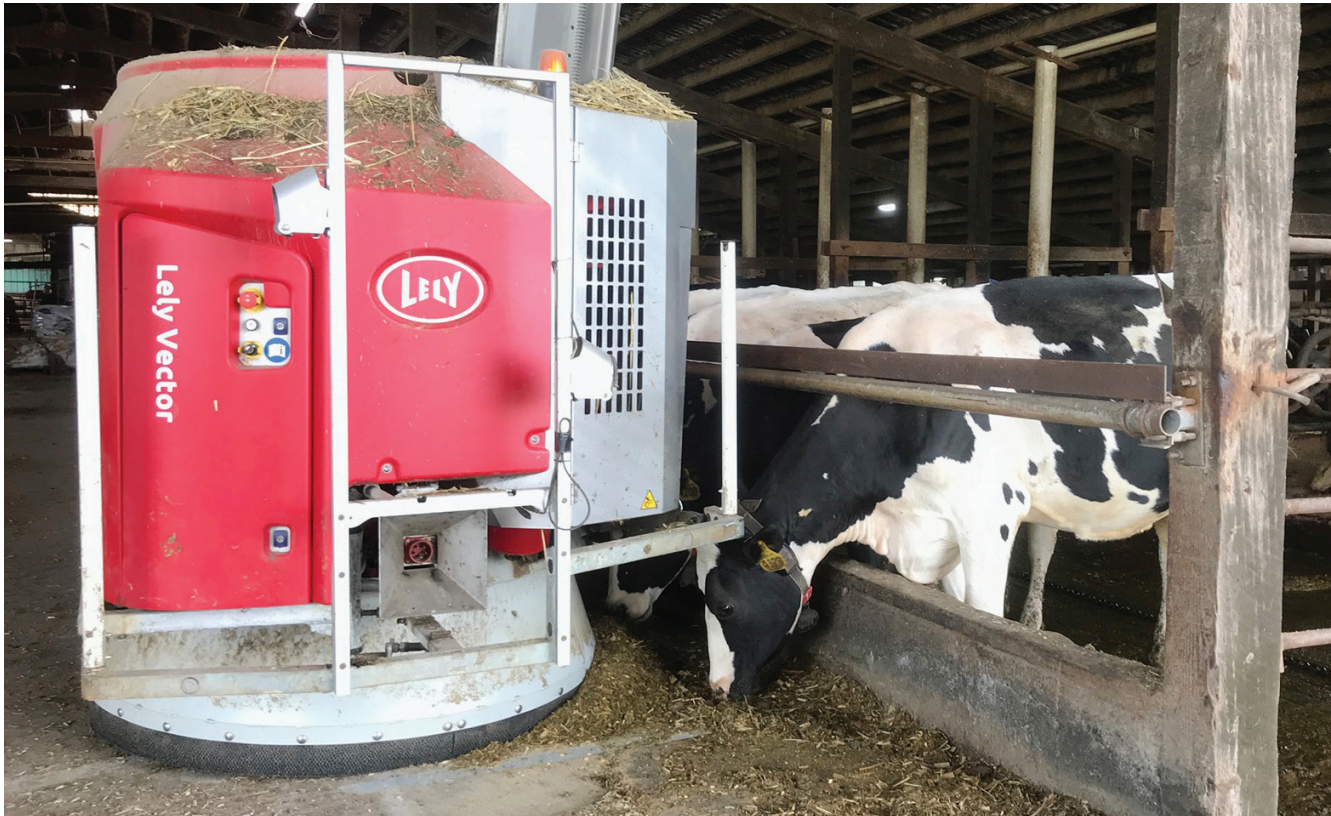
The Lely Vector sweeps along the dairy barn at Tilla-Bay Farms, dispensing a blended mix of feed for 180 dairy cows.
