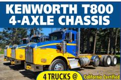
Cummins ISX engines, 18-spd, trans., single spd, Eaton rear-ends 4:10 or 4:11 gears w/locker, HENDRICKSON HAUL-MAX WALKING BEAM SUSP.
