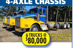
Cummins ISX engines, 18-spd. trans., single spd. Eaton rear-ends 4:10 or 4:11 gears w/locker, **HENDRICKSON HAUL-MAX WALKING BEAM SUSP.**
