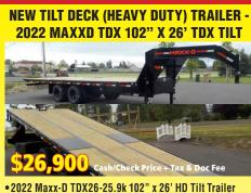
•2 12,000 lb. electric brake axles, 12" X 19 lb. I beam frame with bridge & torque tube., 3" channel cross members on 16" centers, 2 5/16 30k Gooseneck coupler, slipper spring suspension, treated pine deck.
