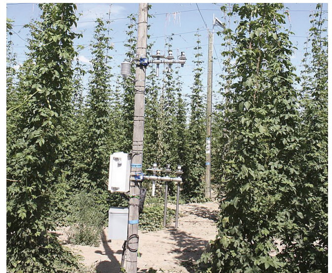
A Washington State University AgWeatherNet system monitors conditions in a hop yard.
