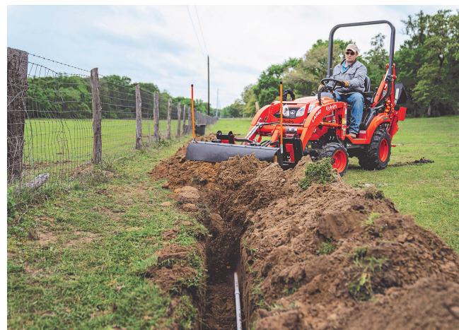
Kubota’s popular BX235 sub-compact diesel tractor takes the labor out of a new water line. No longer than a standard garden tractor, BX Series tractors slip easily between trees and other tight places.
