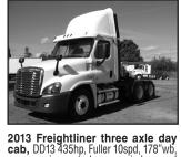
ps, ac, cruise control, power windows and locks, engine brake, air slide 5th wheel dump valve, 352k miles...
