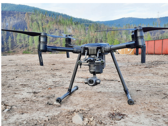
Drone with infrared camera helps Idaho Department of Lands crews monitor fire behavior.
