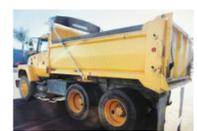
1997 Ford LNT8000 tandem axle dump truck. 14 yard bed. Load tarp. L-10 Cummins with Allison 6 speed auto transmission. PS, AC. Near new Goodyear 11/22.5 radial tires. Former Southern California County truck. Good taxpayer maintenance. Exceptionally clean. NO RUST. Runs drives and operates like new, \$21,000. Located in Twin Falls ID. Call 208-613-0050
