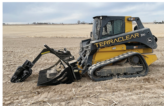
TerraClear's rock picker is used in conjunction with a drone-generated map of all the rocks in a field. The operator follows the map to find each rock.
