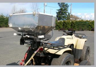
**Bait Spreader**—fast and efficient way to spread baits and minerals
