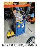
ERCOLINA NEW TUBE BENDER. TB60. BOUGHT FOR CLIENT WHOSE BUSINESS CLOSED. MAX TUBING 1/4" WALL X 2 1/2" DI-AMETER, PIPE MAX 2" SCH40. COMES WITH FULL SET OF TUBING DIES; 3/4", 7/8", 1", 1 1/4", 1 1/2" AND 2". 230
