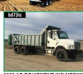
2020 AG EQUIPMENT INC MSP650 Horizontal Manure Spreader Installed on 2010 Freightliner Truck
