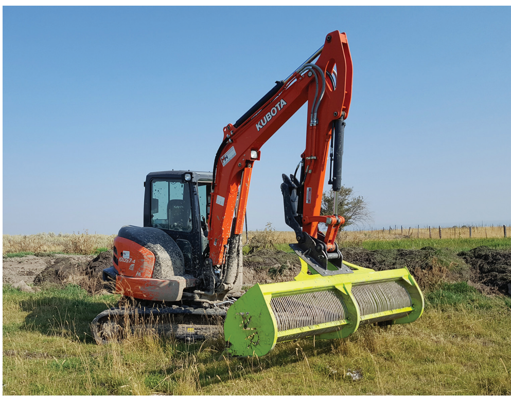
The Aquatic Vegetation Rake attaches to excavators of various sizes and cleans irrigation canals.
