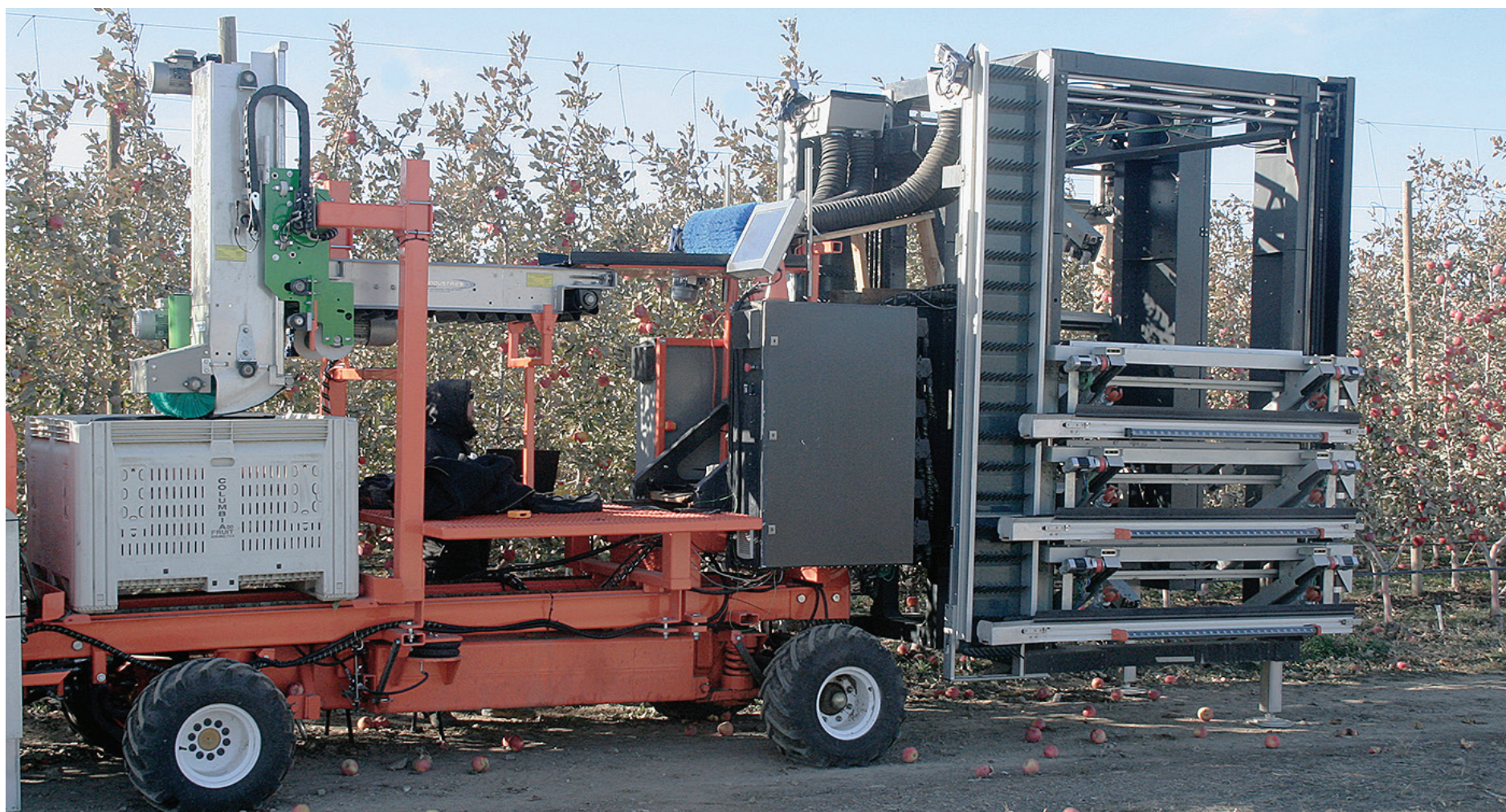
The FFRobotics robotic apple picker mounted on an Automated Ag Bandit Xpress picking platform.
