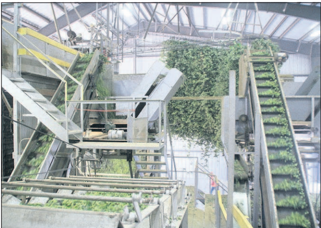
Dan Wheat/Capital Press The new Dauenhauer picking machine at Wenas Hop Co., Yakima, Wash., where hop cones are separated from vines.
