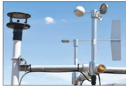
A detailed view of the sensors atop the AgWeatherNet weather stations. The sensors track data related to wind speed, wind direction, air temperature, relative humidity, soil temperature and more.
