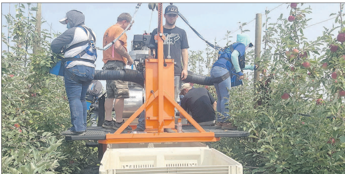
Field testing of Automated Ag-DBR harvest assist in a Stemilt Growers apple orchard in Mattawa, Wash., on July 31. Vacuum tubes replace picking bags. Courtesy of Automated Ag Systems
