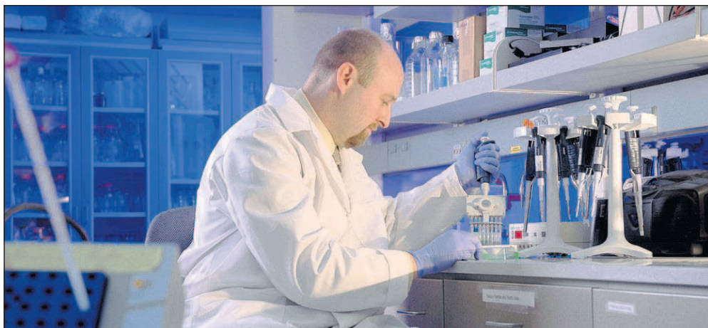
Gordon Murdoch in his molecular laboratory using a multi-channel pipette to analyze specific gene expressions for individual cattle. He said the process can be used in the lab to analyze up to 96 animals at once.
