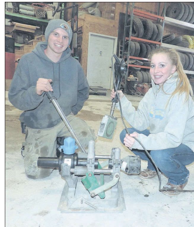
Dianne Troyer/For the Capital Press Jed Heaton's kids, Tykus and Braylee, fuse pipe joints with a McElroy welder.
