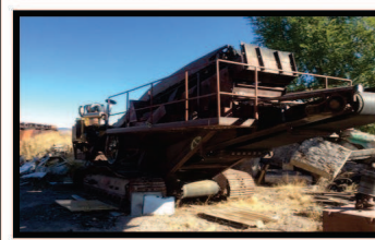
EL-Jay 4125 Track Mounted Crusher w/ KUB-KEN 36X10 Jaw, GM Diesel Pwr.
