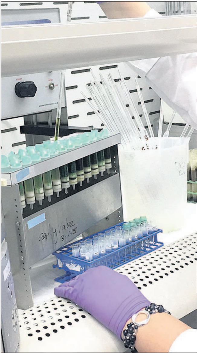
A student worker, Jessica Bowers, performs a solid phase extraction in grass seed straw. This is one of 19 steps in the process of determining the amount of alkaloids in a sample. Testing typically takes four days.
