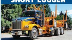
Cummins ISX engines, 18-spd. trans. (RTLO18918B), single spd. Eaton rear-ends 4:10 or 4:11 gears w/locker, HENDRICKSON HAUL-MAX WALKING BEAM SUSPENSION. SHORT LOGGER PACKAGE:
