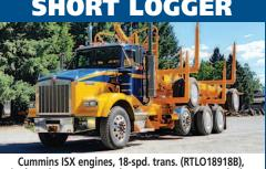
single spd. Eaton rear-ends 4:10 or 4:11 gears w/locker, HENDRICKSON HAUL-MAX WALKING BEAM SUSPENSION. SHORT LOGGER PACKAGE:
