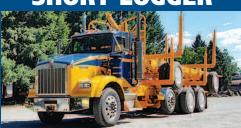
Cummins ISX engines, 18-spd. trans. (RTLO18918B), single spd. Eaton rear-ends 4:10 or 4:11 gears w/locker, HENDRICKSON HAUL-MAX WALKING BEAM SUSPENSION. SHORT LOGGER PACKAGE:
