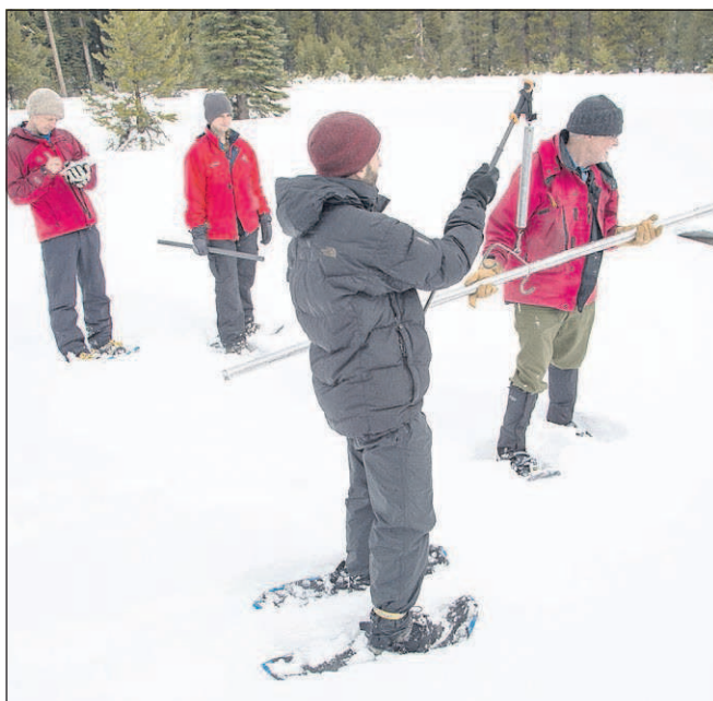
Courtesy of Calif. Dept. of Water Resources From left, scientists Michael Peterson, Julianne McCall and Mikel Shybut assist state snow surveys chief Frank Gehrke with the second manual survey of the 2017 season Feb. 2 at Phillips Station in the Sierra Nevada east of Sacramento.
