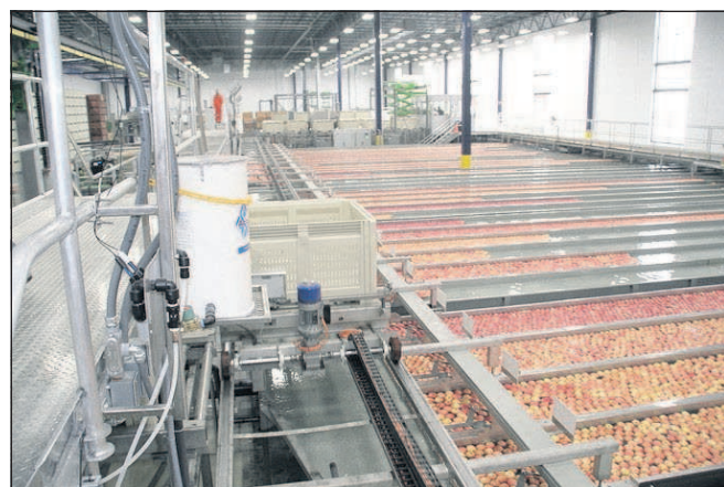
Pre-sized and graded Gala apples await in water lanes for movement into bins for automated movement toward storage at Chelan Fruit Co-op's new plant, Jan. 3.
