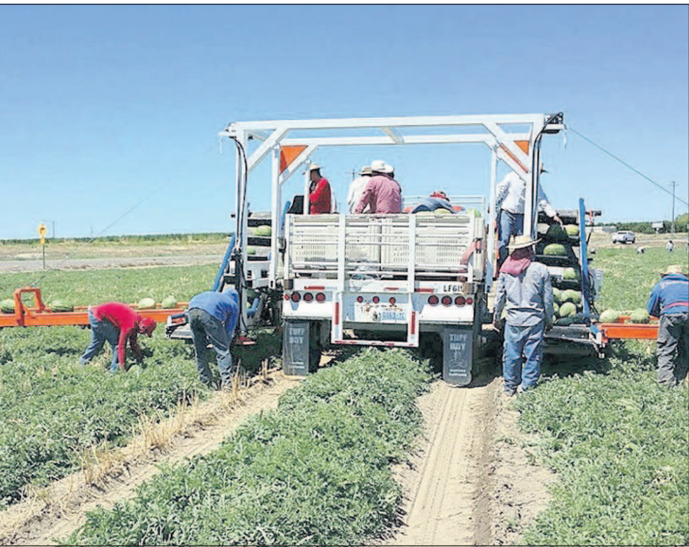
Courtesy of Automated Ag Systems A Melon Wrangler is used to assist workers picking watermelons. The machine can make the job three times more efficient, the manufacturer says.
