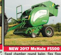
fixed chamber round baler, flex floor, bigger augers, 6.8' pickup, drop floor unblocking system, 15 knife chopper system. #2125 #2126.....\$47,500
