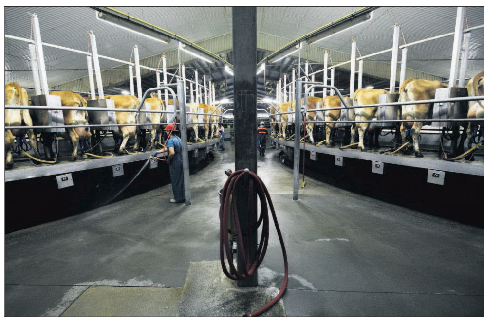
Twin carousels simultaneously milk 80 cows on each side while slowly revolving in the milking parlor at the Columbia River Dairy outside Boardman, Ore.
