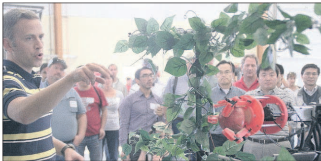
Dan Wheat/Capital Press Joe Davidson, a Washington State University mechanical engineering doctoral student, demonstrates use of a robotic apple picker at a WSU field day in Prosser, Wash., on Sept. 17. Such a device could be a big labor saver for the apple industry.
