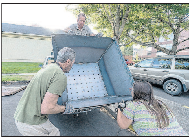
Courtesy of Marcus Kauffman, Oregon Department of Forestry Consultant Kelpie Wilson, right, helps unload a farm-scale biochar kiln during a recent conference at Oregon State University in Corvallis. Welding students at Umpqua Community College have built kilns for a group of farmers experimenting with making and applying biochar.
