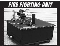
150 Gallon "Econo Model" Wildland Fire Fighter Fiberglass Baffled Tank, CET High Pressure Fire Pump (150 PSI @ 20 GPM) 100' X 1.5" Fire Hose. Excellent Condition & Ready to Work... \$3,250
