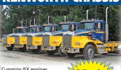
Cummins ISX engines, 18-spd. trans. (RTLO18918B), single spd. Eaton rear-ends 🤜 4:10 or 4:11 gears w/locker, Hendrickson Haul-Max walking beam susp
