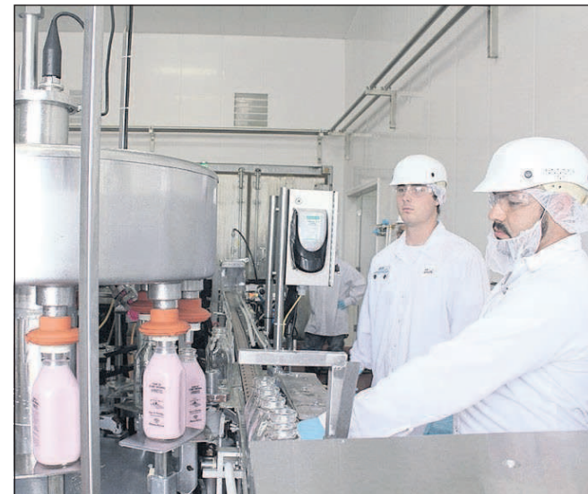
Bottling strawberry-flavored milk at the Top O' The Morn milk processing facility at the dairy.
