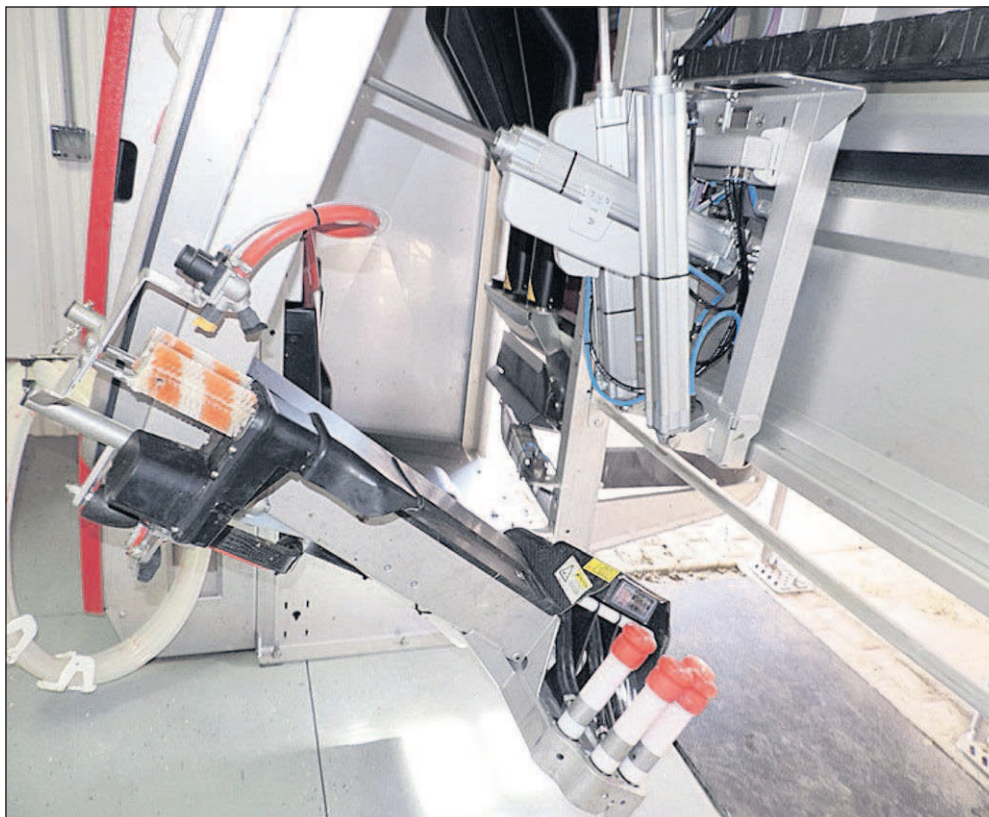
A robotic arm with an optical laser scanner helps locate the teats.
