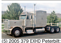
(5) 2005 379 EXHD Peterbilt: 475 HP CAT C-15, 10 speed, 3:55 ratio 404 rear ends with 22.5 rubber on all aluminum wheels. Priced from $33,500 - $43,500. I can remove sleepers for an additional $2,500. Call 509-421-0460
