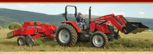
Introducing the 1840 small square baler from Hesston." Thanks to features like its redesigned pick-up, stuffer and exclusive OptiForm™ extended bale chamber, you can count on more capacity, more bale consistency and more uniform density than ever. There's even storage for ten twine spools instead of six. See us soon or go to Hesston.com.
