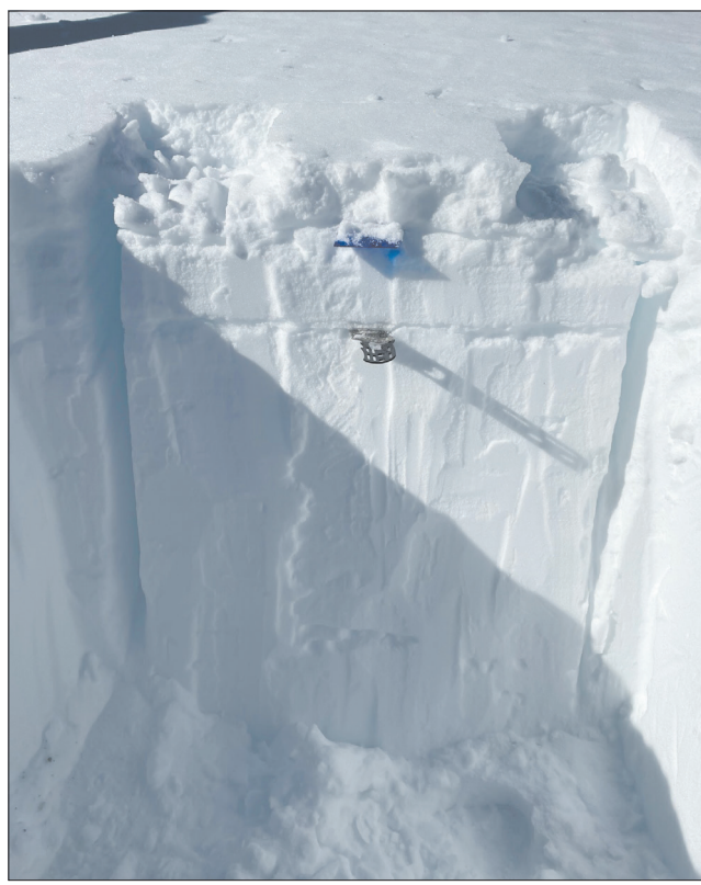
Victor McNeil, director of the Wallowa Avalanche Center, dug this snow pit in the upper Rock Creek area of the Elkhorn Mountains on Jan. 26, 2022. Snow pits allow experts such as McNeil to examine the snowpack for potentially weak layers that raise the risk of avalanches.
