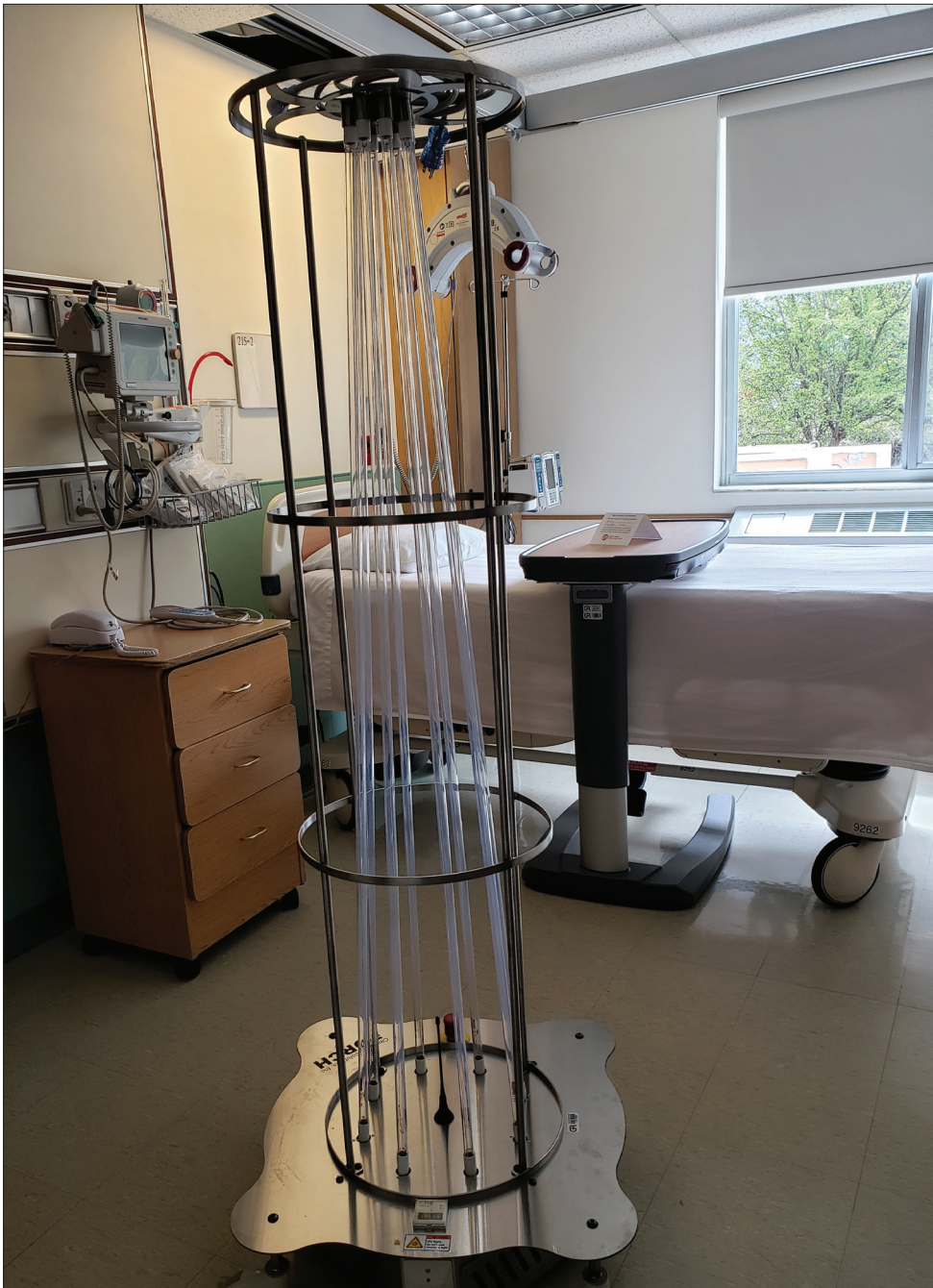
Staff photo by Sabrina Thompson The 6-foot tall "Torch" uses ultraviolet light to disinfect rooms throughout Grande Ronde Hospital. The light disinfects surfaces in 15 minutes.
