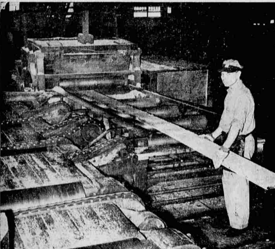
THE EDGER: Still more sawing. Here Ben Kramer, the edger, takes the rough edges off the rough boards and has to decide quickly also as to the cuts to be made.
