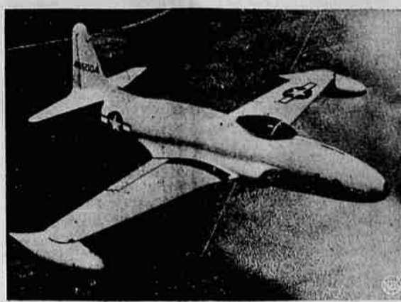
PLANE WHICH CARRIED Maj. Richard Bong to his death is this type of P-80 "Shooting Star," jet propelled. It does better than 550 m.p.h. and its ceiling is more than 40,000 feet.
