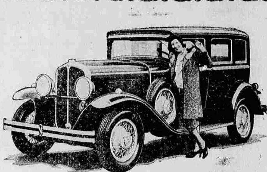
New peaks of power, speed and acceleration feature the new Oakland Eight. It is powered with a sturdy, compact, 90-degree V-type eight-cylinder motor employing many new but thoroughly proved principles of design. Shown here is the New Oakland Eight 4-door sedan.
