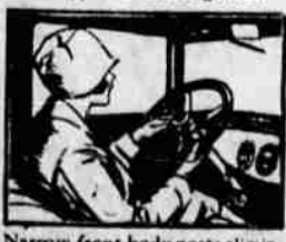
Narrow front body post eliminates the "blind spot" hazard and permit clearer vision.
