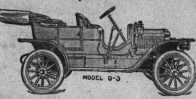
This model is a small five passenger touring car with 22 H. P., equipped with sliding gear transmission. A car for the man with a small family and it is a popular seller SALE PRICE ...... \$1200
