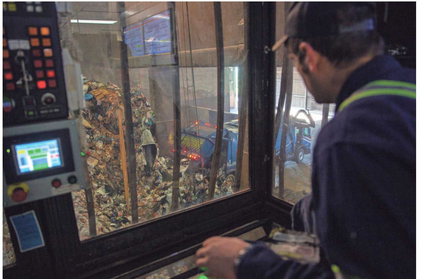
Covanta employee Brad Berkey, an auxiliary operator, sorts garbage deposited by local trash haulers at Covanta Marion, Inc. in Brooks, Ore. on Dec. 5. The Energy-from-Waste facility processes on average 550 tons per day of municipal solid waste (MSW) from Marion County. MADELEINE COOK / STATESMAN JOURNAL
