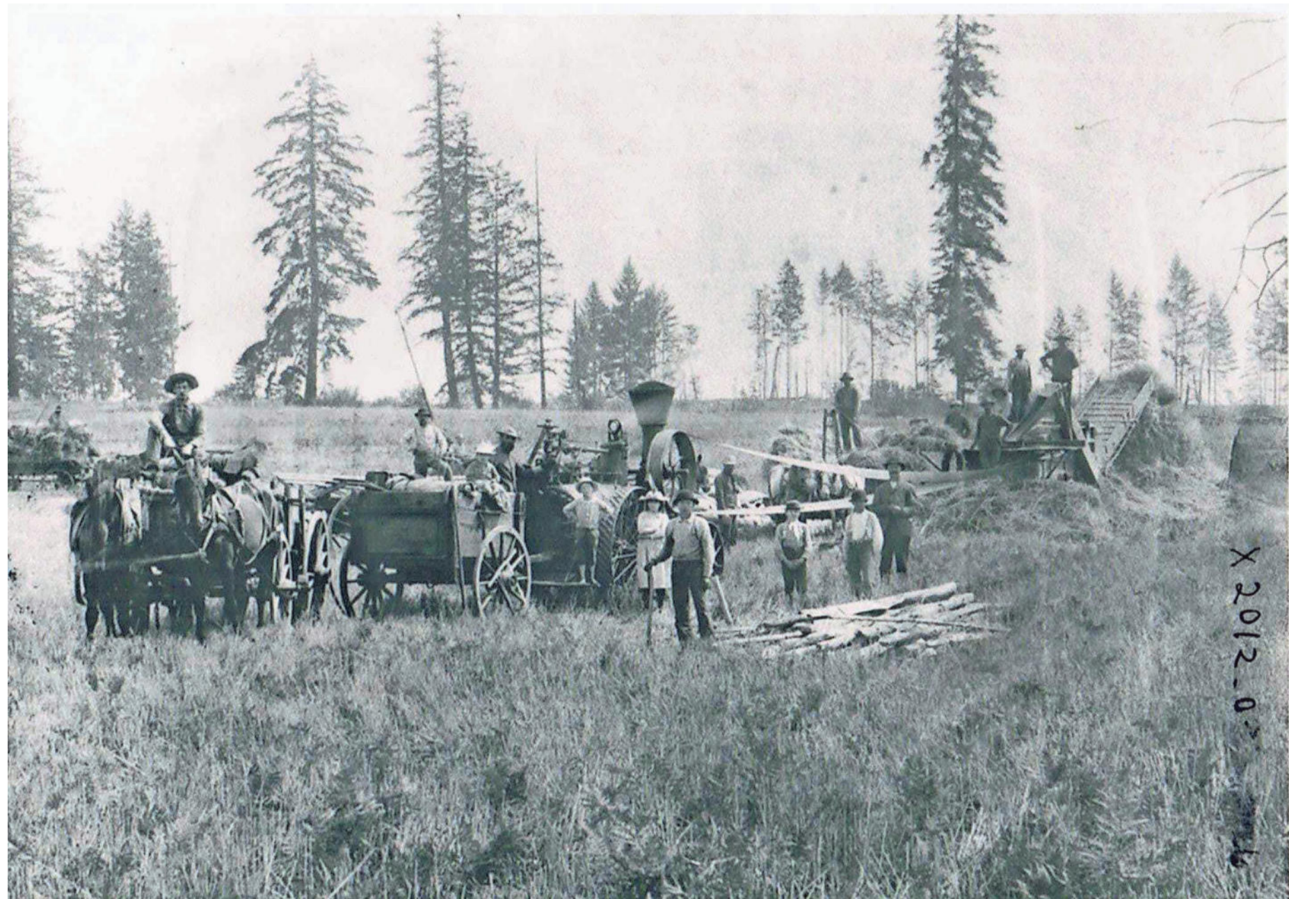
Steam engine belted up to a threshing machine at what now the 2600 block of Summer St. SE in Salem in 1894. Scenes like these were common summer sights in the Salem area in the late 19th and early 20th century. WILLAMETTE HERITAGE COLLECTIONS
