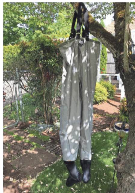
To find leaks in your waders, hang them from a tree and fill with water.
